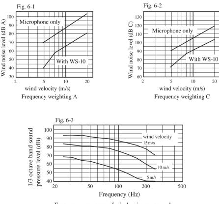
Frequency response of wind noise measured with windscreen WS-10 mounted microphone
