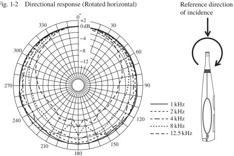
Fig. 1-2 Directional response (Rotated horizontal)
