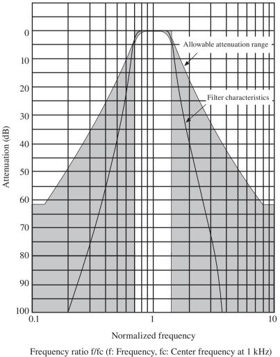
Attenuation tolerance according to IEC 61260:1995 class 1 and octave band filter characteristics of NA-28
