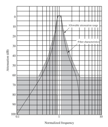
Frequency ratio f/fc (f: Frequency, fc: Center frequency at 1 kHz) Attenuation tolerance according to IEC 61260:1995 class 1 and 1/3 octave band filter characteristics of NA-28
