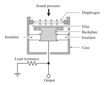
Construction of prepolarized condenser microphone
