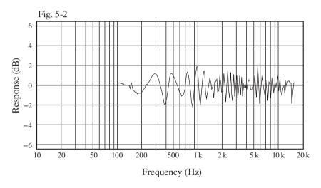
Acoustical influence of operator (the distance from the top of the microphone to the operator is approx. 70 cm)
